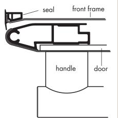
When securing the appliance, the fixing screws provided are driven through the edging strips into the cabinet - the seal will straighten up and sit flush to the cabinet when the screws are fully home.
