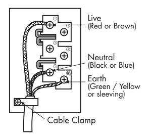
Minimum cable thickness must be  $6mm^2$ .
