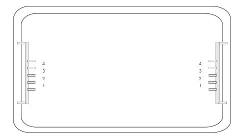
The top oven and grill has 4 shelf positions which are counted from bottom to top. You can also adjust the positioning of food by turning the grid in your grill pan. The cooking guides in this handbook are accompanied by a recommended shelf position see page 29 for details on grilling and page 36 for details on the top oven.
