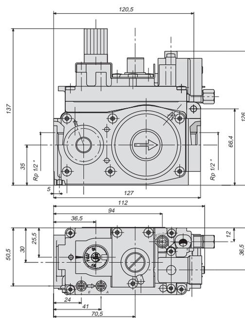
Multi-functional gas valve with On-Off gas flow control suitable for use with boilers, catering equipment, furnaces, radiant tubes and space heaters. SIT 820 NOVA is available in AC-powered versions (220/240V or 24V) or versions powered by a millivolt generator which permits complete control of the appliance without requiring main supply voltage. All versions are available, on request, with manual adjustment of the gas flow.
